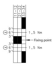
Point of fixation is in range of  $0^{\circ}$  ...  $270^{\circ}$  free selectable.
